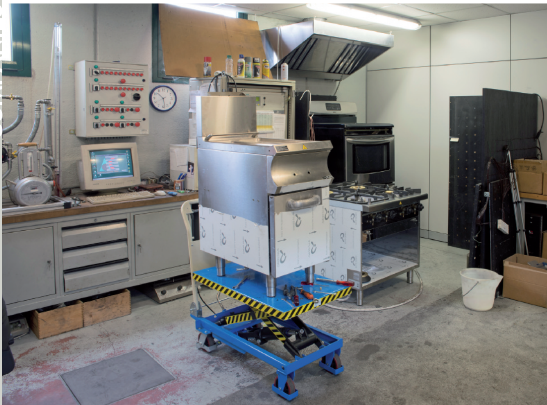
Actek laboratory, equipped according to EN30, EN203 and EN60335 regulations, can test and approve customers' products.
